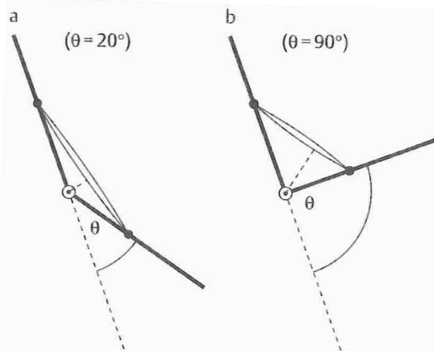
During flexion of the joint, the arm lever of the muscular force varies. If we need to maximise the muscular force to lift an heavy object, it would be more effective to start the motion with the joint having a  $90^\circ$  flexion as shown on the example given here.
